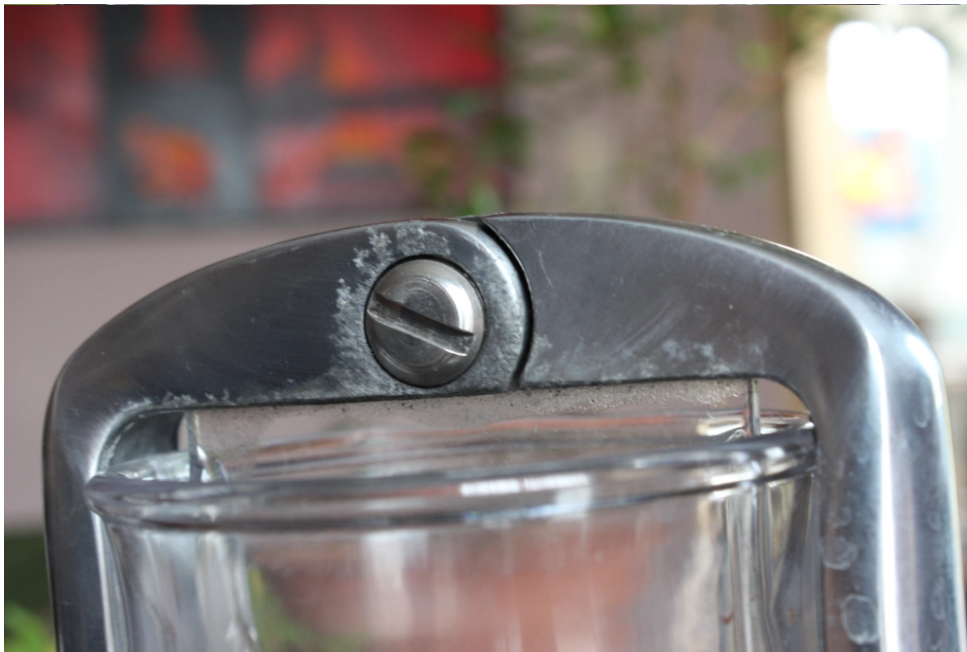
( https://artofolivegreen.files.wordpress.com/2013/03/img_2060.jpg ) Galvanic corrosion around the joint.
