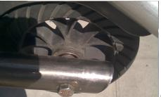
(https://artofolivegreen.files.wordpress.com/2012/08/imag1740.jpg) There should be a blue plastic wall fused between the collar and outer edge of the roller bearing.
